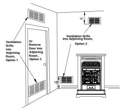
Figure 2-Ventilation Air from Inside Building
